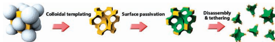
Figure 1. Schematic diagrams illustrating the processing steps to produce end-functionalized tetrapods.
